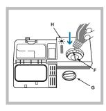
Open the dispenser by turning the lid (G) in an anticlockwise direction.
